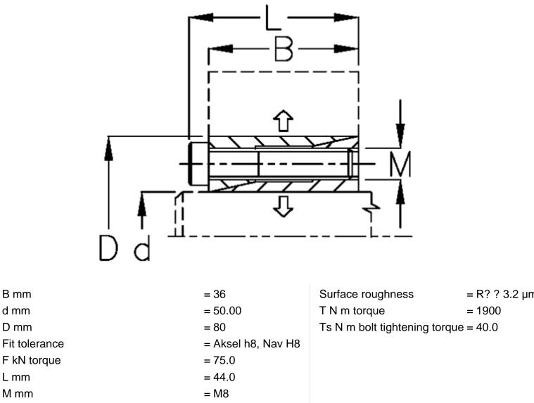
P N/mm2 surface pressure on shaft/hub = 115
